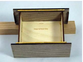
Next, sand the face of the two keyway pieces with 180/220 grit sandpaper to make it easier for the holder panel to slide over it. Then, using the blue (.220") pegs, glue the left end keyway to the left box end and the right end keyway to the right box end.
