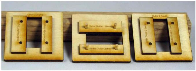
After the glue is dry, sand the outside face of each piece with 180/220 sandpaper. I then applied clear finish just to the outside face.
