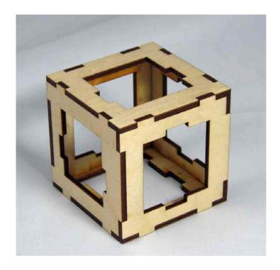
After two/three coats of finish I dis-assemble the box. The purpose of applying the finish with the box put together like this is to prevent getting finish on the edges of the box panels that will need to be glued later. After the finish dries on these pieces, test fit the Outer 1 panel assemblies with the appropriate Outer panel pieces to make sure the Outer 1 piece slides smoothly. When looking at the pieces from the inside, the writing on the pieces should be oriented in the same direction.
