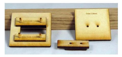
Insert the slider assembly into the inside of the Outer 1 (base) panel and then glue the Outer 2 (base) panel to the slider assembly.
