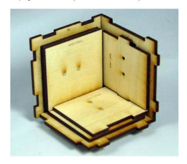
With the Outer 1 and Outer 2 panels centered, glue on the right side and then glue on the back side. The Base box panel can then be glued in place.
