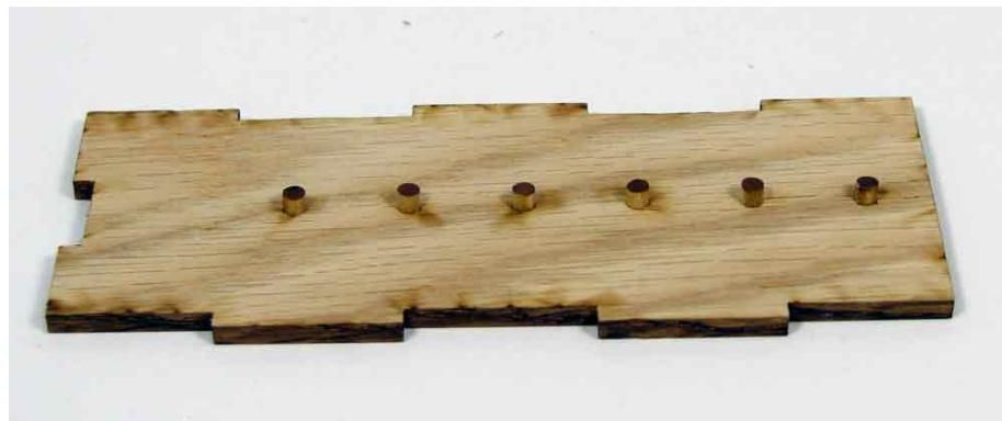
You could put glue on each of the pegs before inserting them or you can go back after they have all been inserted and put a drop of super glue on the inner side of the pegs to lock them in place as shown below.
