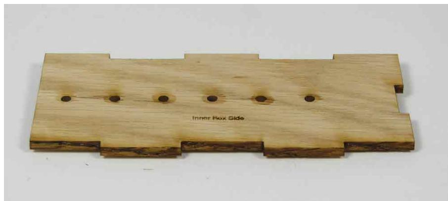
Next glue the front, left, back, right and bottom panels of the inner box together. The writing on the side panels should be facing inwards and the writing on the bottom panel should face towards the inside of the box.
