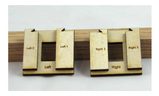
The pieces should be flush/even with the top of the panel and the side of the panel. After these are dry test the fit of the left/right 2 pieces between the 1 & 3 pieces. It should slide freely. If not, use sandpaper to lightly sand the edges until it moves easily.
