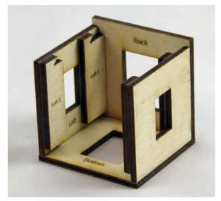
After the glue dries, slide the inner bottom panel into place. If this piece does not slide freely, work it back and forth or slightly sand the edges until it does. Sanding the sides that slide against each other and waxing them makes pieces move better. Sanding a slight bevel around the bottom edge of the inner panel also helps.
