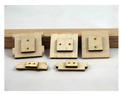
Place the front, left, back and right side slider assemblies into the box and make sure they still slide freely. You may need to bevel the edges of the inner sliders where they pass next to another inner slider to get them to move smoothly.
