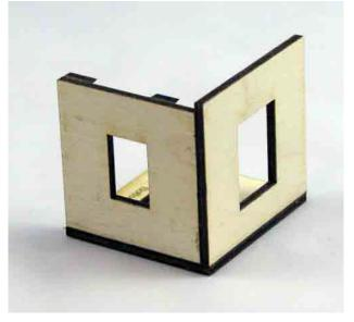
Now glue the left panel to this assembly. Use the bottom inner panel and the back panel as spacers for positioning the left panel, but remove them quickly otherwise they will get glues in place (you could put some
