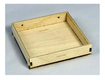
Glue the two stop support pieces to the back side of the drawer using the green (.370") pegs. Then glue the drawer stop onto those two pieces. After the glue has dried sand all sides smooth and test fit it in the box assembly. If it binds then sand the area of the bind until it moves smoothly.
