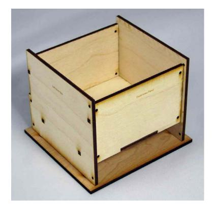
After the glue is dry sand the four sides of the box with 100 grit sandpaper to remove any ridges and make it smooth for any sliding pieces.
