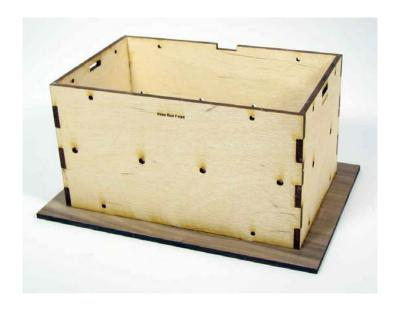
After the glue is dry sand the four sides of the box with 100 grit sandpaper to remove any ridges and make it smooth for any sliding pieces.
