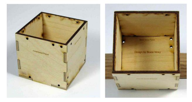
After the glue is dry sand the four sides of the box with 100 grit sandpaper to remove any ridges and make it smooth for any sliding pieces. Then sand it with 180/220 grit sandpaper to make it really smooth for the sliding panels.
