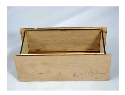
Make sure to remove any glue squeeze out before it dries. After the glue has dried glue the lower inner ends for both the left and right sides. After the glue has dries test fit the false bottom panel and the inner lid panel. Sand or file these pieces to make sure they slide smoothly. Finish sand the base, front and back sides now since it is easier before the base is glue onto the box. Glue the base piece to the box assembly.
