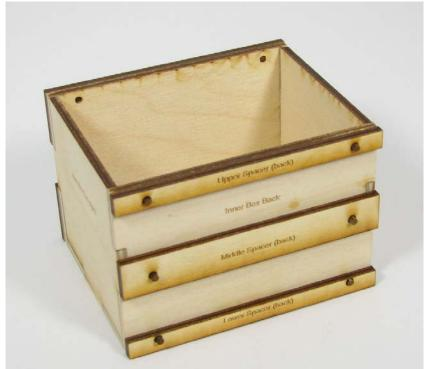
After the glue has dried check the fit of the front and back slider holders. Make sure that they slide smoothly between the spacer pieces.
