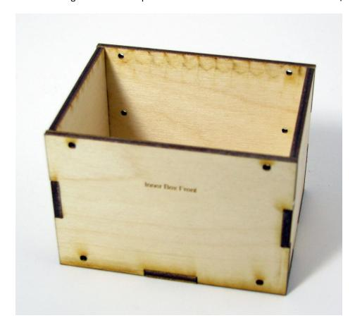
After the glue is dry sand the four sides of the box with 100 grit sandpaper to remove any ridges and make it smooth for any sliding pieces. Then sand it with 180/220 grit sandpaper to make it really smooth for the sliding panels.
