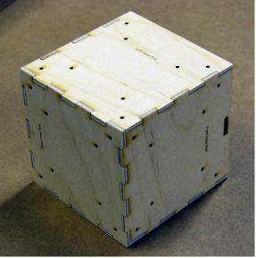
After the glue has dried sand outside faces of the inner box to make smooth and remove any ridges (100 grit). This is best done by taping the sandpaper down to a hard flat surface and then moving the box over the sandpaper. This is shown in the photo below.
