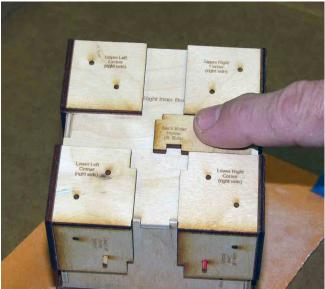
Perform the test fitting for all of the slider holders on each face of the box. Another step that you can take to prevent the slider holders from catching is to bevel the back edge of the slider holder that extends over the corner of the box.
