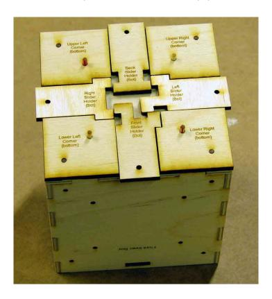
To prevent the slider holders from binding when the outer panels are attached you can sand down the back slightly to make them a hair thinner. Do this by sanding the slider holders with about a half dozen strokes on the sandpaper laying on a hard flat surface as shown in the following photo. After sanding, a little paraffin or candle wax can be applied to the back of the slider holder and then worked into the wood by sliding back and forth on the box as shown in the photo on the right.
