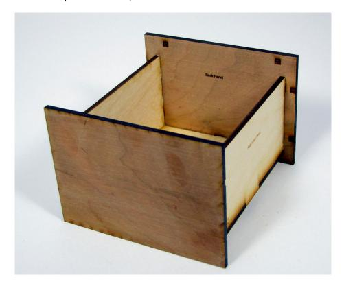
After the glue is dry sand the left, right and bottom inner sides of the box with 100 grit sandpaper to remove any ridges and make it smooth for any sliding pieces. Then sand it with 180/220 grit sandpaper to make it really smooth for the sliding panels.
