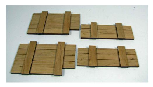
Make sure that after both cross strips have been glued that you place this assembly on a flat surface with the cross strips down. Then make sure that all the long/dummy strips are pressed firmly down onto the cross strips. The pegs may still stick out of the inner side (the side that is now facing up), but these will be sanded down in the next step.
