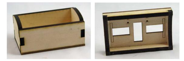
After the glue has dried sand the sides of the box and lid with 100 grit sandpaper. I lay the sandpaper sheet on a flat hard surface and then move the piece I am sanding over this (see photo below). I also have found that it is best to hold the lid and bottom together while sanding to make sure the outsides of the box/lid are flush with each other. After sanding the box and lid, it should look like the box below on the right.
